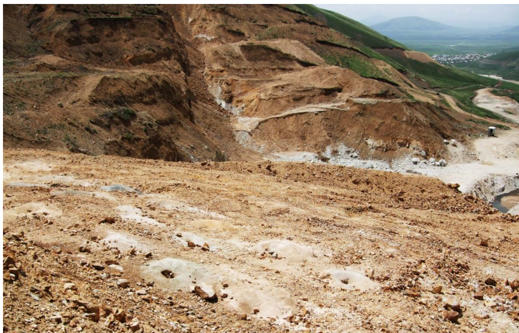
Figure 31 Bench blast holes completed in advance of mining in Toukhmanuk pit
