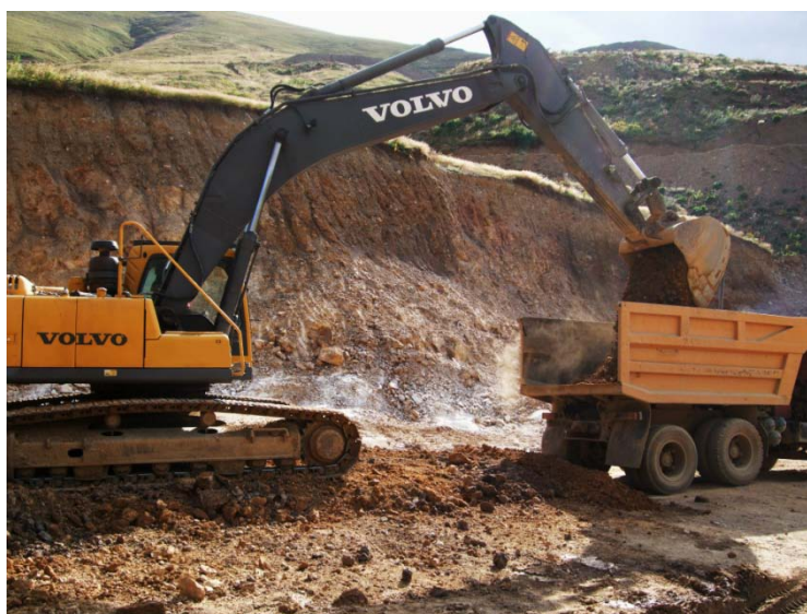
Figure 52 Tracked shovel loading truck in Toukhmanuk pit Notice shallow soil profile behind shovel arm this is reported to be stockpiled for use in later mine rehabilitation
