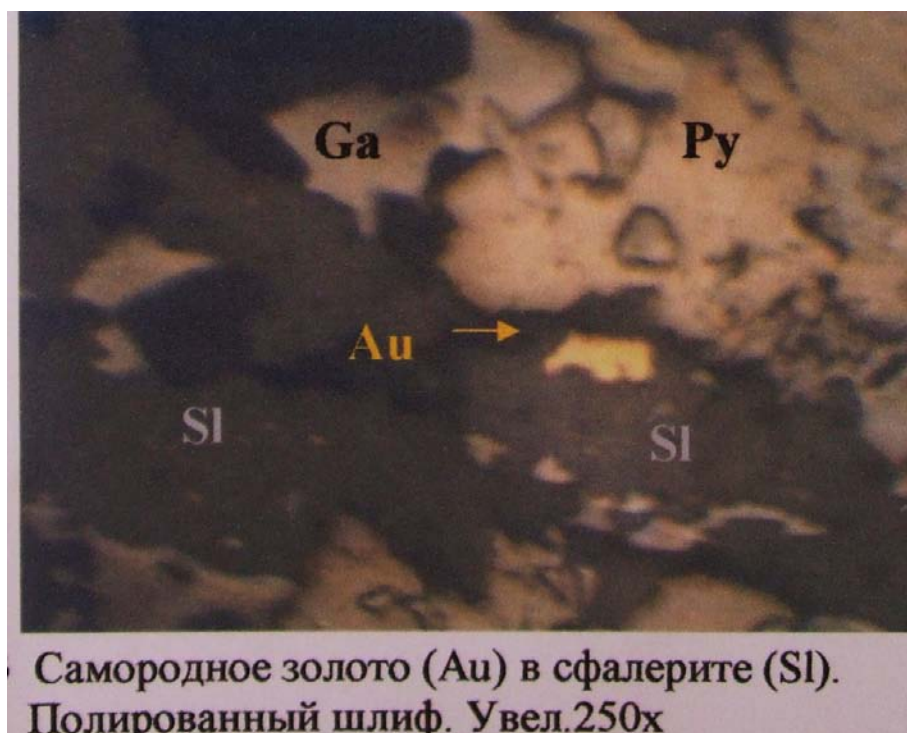
Figure 44 Sphalerite with encapsulated gold corroding pyrite and galena, Toukhmanuk
