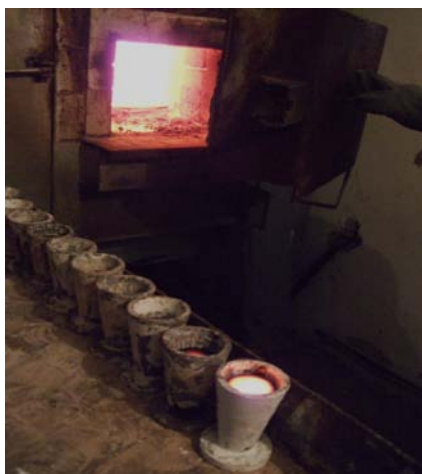
Figure 22 Cupels cooling after removal from the gold room furnace, Toukhmanuk
