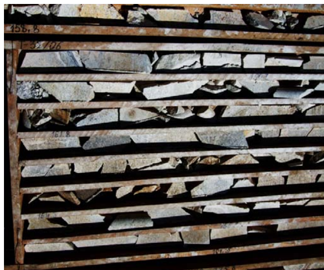
Figure 40 Representative stored drill core, hole T 32, drilled in 2006 159.8 m to 167.5 m depth, with examples of mineralized veins in quartz porphyry.
